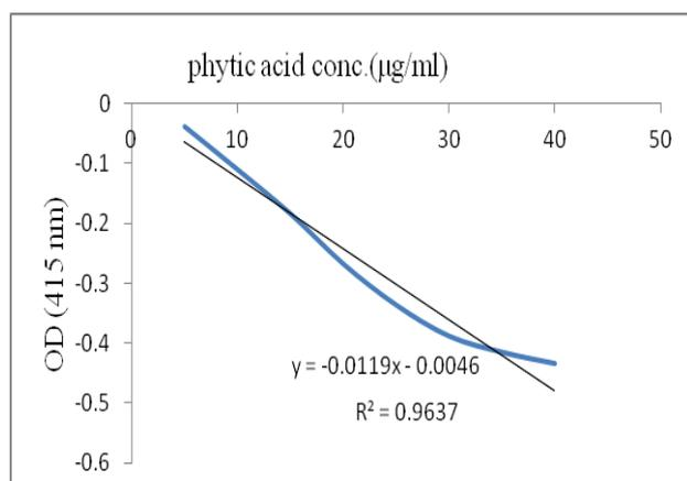
Figure 1. Standard curve of phytic acid
